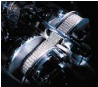
Cutaway of Audi's CVT showing the variable-diameter pulleys that replace the conventional gearset
