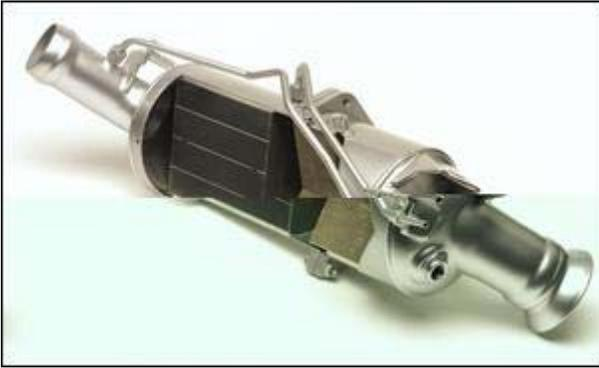
Exhaust particulate filters are made from porous ceramic materials. When they become full, they can be regenerated by being heated to above 600 degrees C. This is a higher exhaust gas temperature than is normally experienced in diesels and to achieve this, retarded injection and intake flow restriction can be used to increase the temperature of the exhaust gas.
