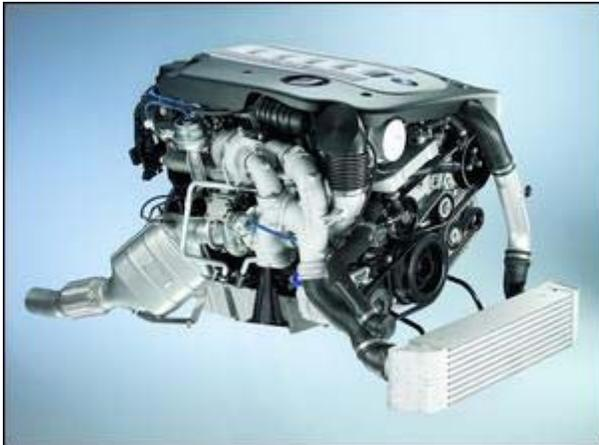
Although the basic designs of petrol and diesel engines are similar (both are two or four stroke designs which use reciprocating pistons driving a crankshaft), a diesel engine does not compress its fuel/air charge and then initiate combustion by the use of a spark plug. Instead, in a diesel engine just air is compressed. When the piston is near Top Dead Centre, the fuel is sprayed by an injector into the combustion chamber, whereupon it mixes with the hot compressed air and self-ignites.
